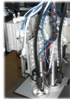
VALVES IN AUTOMATIC PURGE PROCESS
