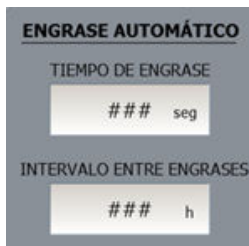
AUTOLUB SYSTEM CONTROL WINDOW
